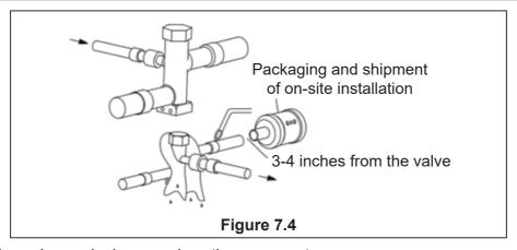
5. After the service valve cools down, replace the pressure tap.
