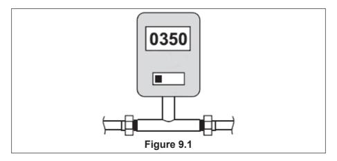
2. Observe micrometer gauge. If the micrometer meter does not rise above 500 micrometers within one (1) minute, the evacuation is completed.
