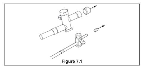
2. Remove the pressure taps from the two service valves.
