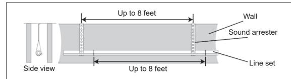
Use isolators to fix the suction line every 8 feet. Every 8 feet, liquid line directly to the suction line with tape, wire or other suitable methods.
