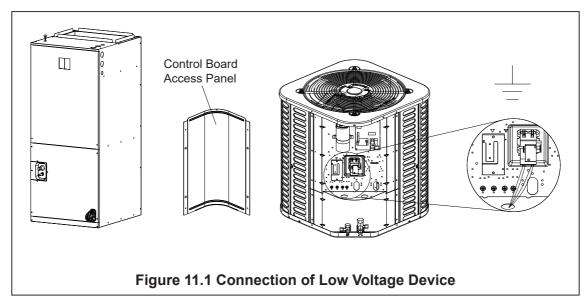
**NOTE:** The reference figure shows the selection of the low voltage wire hole of the 60K model, and the selection of the wire hole of other models should be made according to the national, state and local regulations.
