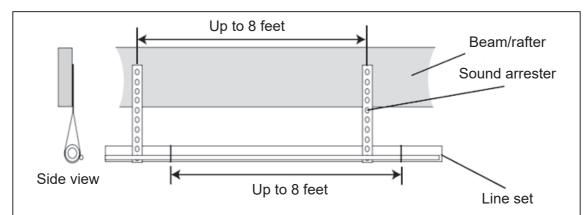
Use isolators to fix the air pipes on the beams every 8 feet. Every 8 feet, tape, wire or other suitable methods are used to fix the liquid line directly to the suction line.
