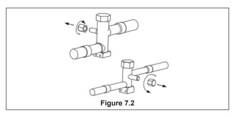
3. Purge refrigerant lines and indoor coils with dry nitrogen.
