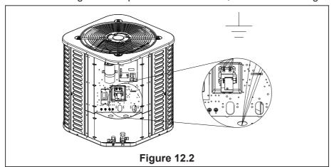
**NOTE:** The reference figure shows the selection of the high voltage wire hole of the 60K model, and the selection of the wire hole of other models should be made according to the national, state and local regulations.
