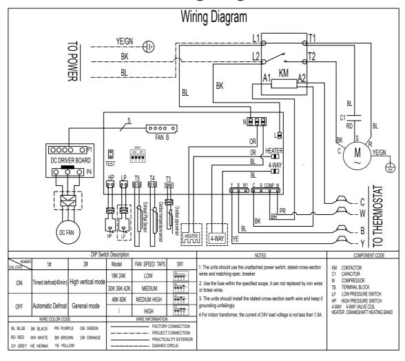
NOTE: For reference only, the actual wiring diagram shall prevail
